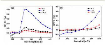
Fig. 5 IPCE measurements at (a) fixed applied potential 1 V and (b) fixed wavelength 350 nm.
