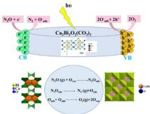
Fig. 7 Plausible mechanism for photocatalytic decomposition of N<sub>2</sub>O using Bi-based photocatalysts
