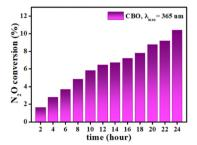
Fig. 6 Time dependence on the N<sub>2</sub>O conversion during the photocatalytic decomposition of N<sub>2</sub>O over CBO under UV-A irradiation at 365 nm.
