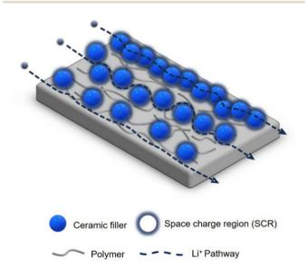
Fig. 1 Illustration of the three proposed main mechanisms of Li ion migration through a composite polymer electrolyte (CPE) composed of a polymer matrix and ceramic filler particles.
