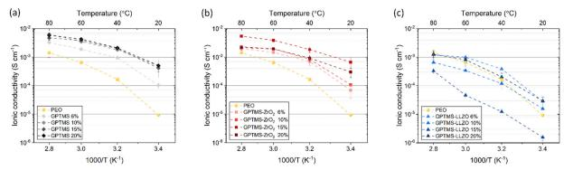
Fig. 6 Ionic conductivity of 6, 10, 15, 20 vol% of (a) GPTMS CPE, (b) GPTMS-ZrO<sub>2</sub> CPE and (c) GPTMS-LLZO CPE measured at 20, 40, 60, and 80 °C in comparison of PEO SE.
