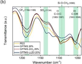
Fig. 4 (a) The second heating curves of the DSC measurements and (b) FT-IR spectra of the PEO-LiTFSI SE, filler-free GPTMS 20% CPE, GPTMS-ZrO $_2$  20% CPE, and GPTMS-LLZO 20% CPE.
