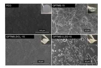
Fig. 9 SEM images and digital photos (top right) of PEO SPE with smooth surface, GPTMS 15% CPE with fibrous and uneven structure, GPTMS–ZrO $_2$ 15% CPE with homogeneous surface and a uniform distribution of particles, and GPTMS–LLZO 15% CPE with heterogeneous surface and large particle agglomerates.
