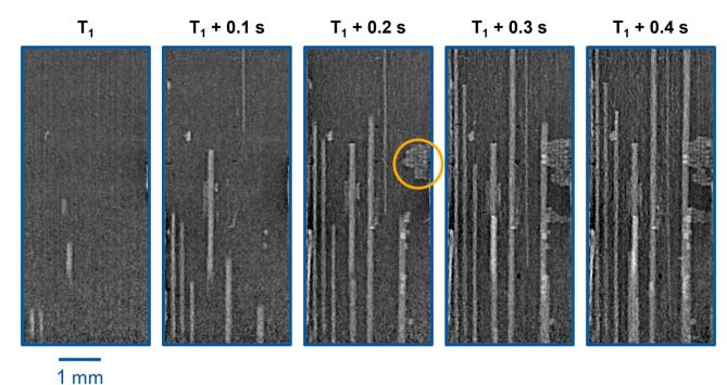
Fig. 5 Sequence of representative radiographs selected from synchrotron X-ray in situ 2D radiography experiment showing electrolyte injection in the
