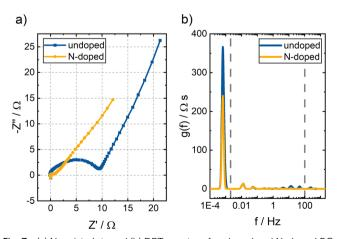
Fig. 7 (a) Nyquist plots and (b) DRT spectra of undoped and N-doped BC. A V(IV) electrolyte and a flow rate of 15 mL min<sup>-1</sup> were used. A potential of 1.05 V vs. RHE was applied.
