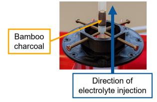
Fig. 2 Measurement setup for injection experiments with a synchrotron X-ray beam.
