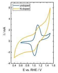
Fig. 8 CV of undoped and N-doped BC at a scan rate of 2 mV s<sup>-1</sup> in V(IV) electrolyte
