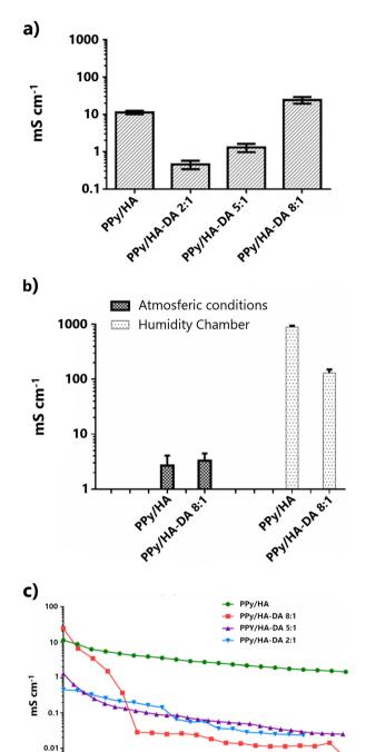
**\*\*Meformation\*\***Fig. 13 (a) Conductivities of PPy/HA and PPy/(HA–DA) films on a poly(dimethylsiloxane) substrate. (b) Conductivities of PPy/HA and PPy/(HA–DA) 8:1 films under different humidity conditions. (c) Conductivity as a function of applied stress; conductivity measurements are shown as the mean and standard deviation of n=3. Reproduced, with adaptations, from ref. 233 with permission from Elsevier; copyright © 2017 Elsevier B.V.
