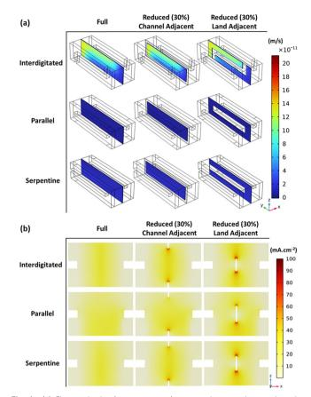
Fig. 4 (a) Flow velocity (x component) across the membrane domains for MEAs with full membrane coverage or 30% channel/land adjacent membrane reduction. (b) Electrolyte current density profiles for the flowfield designs of the full membrane coverage and 30% reduced membrane coverage architectures. The negative electrode is on the left, positive on the right.
