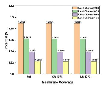
Fig. 5 (a) Steady-state discharge polarization of cells adopting interdigitated at 50% SOC and 100 mA cm<sup>-2</sup>. Showing full membrane coverage and 10% total membrane coverage reduction – adjacent to channel or land. CR: Channel-adjacent membrane reduction MEA architecture, LR: land-adjacent membrane reduction MEA architecture.
