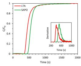
Fig. 8  $CO_2$  breakthrough curves of the LTA and SAPO-34 beads. The inset displays the derivative of the breakthrough curves. Feed: 40 vol%  $CO_2$  and 60 vol%  $CH_4$  (mimicking biogas).
