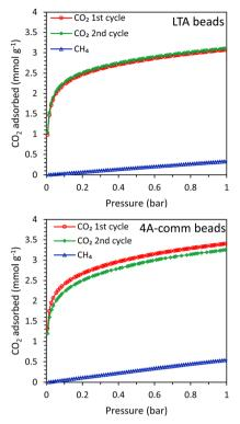
Fig. 3 CO<sub>2</sub> (2 cycles) and CH<sub>4</sub> adsorption isotherms of the LTA beads (top) and 4A-comm beads (bottom)
