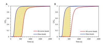
Fig. 2 (A) Area between the breakthrough curve of the glass beads and that of the adsorbent (yellow) for  $CO_2$  adsorption capacity at full utilization; (B) area between the vertical line from the breakthrough time,  $t_{\rm b}$ , and the breakthrough curve of the glass beads (yellow) for  $CO_2$  adsorption capacity at breakthrough.
