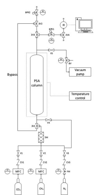
Fig. 1 Schematic overview of the experimental setup for conducting VPSA breakthrough experiments. V = valve; 3V = three-way valve; BV = bleeding valve (regulating the reduced pressure); CV = check valve (preventing back-flow); FI = flow indicator; FM = variable area flowmeter; MFC = mass flow controller; SM = static mixer; BPR = back pressure regulator; PI = pressure indicator; IR = infrared CO<sub>2</sub> sensor.
