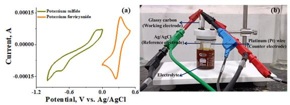
Fig. 6 (a) Cyclic voltammogram of potassium sulfide and potassium ferricyanide at 10 mV s<sup>-1</sup> and (b) digital photograph of the three-electrode experiment assembly.
