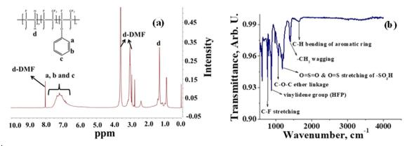
Fig. 2 (a) <sup>1</sup>H-NMR spectra of phenol-docked-PVDF-co-HFP polymer and (b) FT-ATR spectra of the T-CEM
