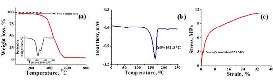
Fig. 3 Thermal and mechanical stability evaluation of the T-CEM. (a) TGA spectra; inset figure: first order derivative graph. (b) Differential scanning calorimetry (DSC) spectra and (c) universal testing machine (UTM) analysis of the T-CEM.
