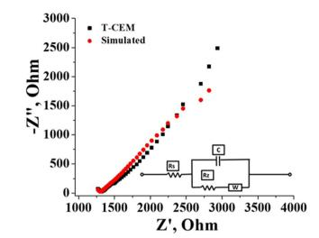
**Fig. 5** Impedance spectra of the T-CEM with simulation; inset figure: Circuit diagram.
