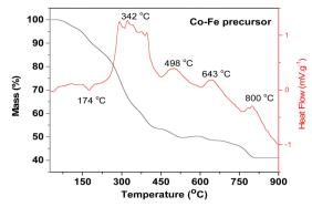
Fig. 2 Thermogravimetric (TGA) curve for the Co-Fe precursor.
