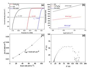
Fig. 7 (a) LSV curve of CoFe<sub>2</sub>O<sub>4</sub>. (b) Tafel plot of CoFe<sub>2</sub>O<sub>4</sub>. (c) C<sub>dl</sub> plot of CoFe<sub>2</sub>O<sub>4</sub> obtained from the cyclic voltammetric curve at different sweep speeds. (d) Nyquist plot of CoFe<sub>2</sub>O<sub>4</sub>
