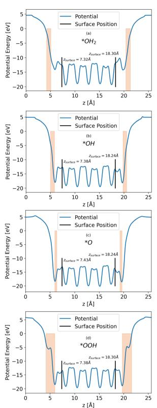
Fig. 2 x-y averaged potential of the (a) \*OH<sub>2</sub>, (b) \*OH, (c) \*O, (d) \*OOH intermediates (from top to bottom, respectively). The black lines in each graph represents the location of the bottom and top surfaces of the slab. Intermediate positions are shown in the orange shade.
