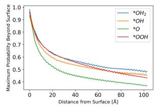
Fig. 6 Probability to reach the surface by starting distance, from egn (31) with different starting  $z_0$  values.
