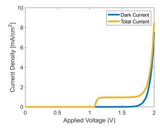
Fig. 7 Simulated J-V curves with and without photocurrent.
