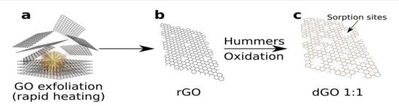
Fig. 7 Scheme for the preparation of defective GO: (a) explosive thermal-exfoliation of GO, (b) Hummer's oxidation of defective rGO and (c) dGO with sorption sites.219
