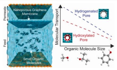
Illustration of the performance of the NPG membrane for the removal of organic molecules.<sup>229</sup>
