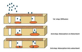
Fig. 3 Mechanism of classical adsorption.
