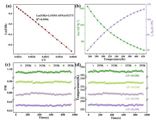
Fig. 9 (a) The relationship between Ln(FIR) and 1/T. (b) Absolute sensitivity and relative sensitivity of (KMg)ScW<sub>3</sub>O<sub>12</sub> phosphor dependence on temperature. (c) Calculated FIR values at 293 K, 313 K, 333 K and 353 K. (d) Corresponding temperature and ΔT recorded at 293 K, 313 K, 333 K and 353 K.
