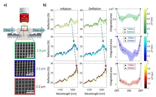
Fig. 4 Analysis of pressure variation detection by monitoring changes in optical properties for WD periodicities. (a) In situ pressure bulge setup for measuring the optical properties of WDs with 1.9 (green), 2.1 (blue), and 2.2 µm (red) periodicities. (b) Reflection spectra of three periodicities recorded during inflation (left) and deflation (middle) and the resulting pressure sensitivity performance (right). Faded colours stand for measurement errors. Arrows indicate the resonance position.
