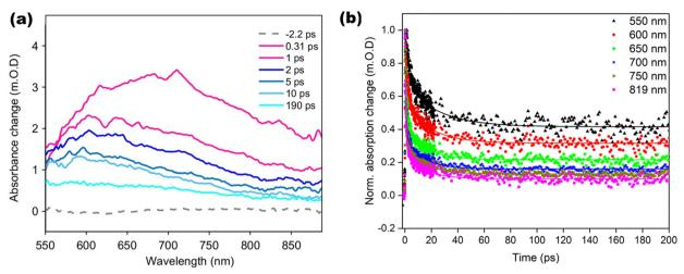
Fig. 6 Time-resolved broadband TAS spectra and TAS relaxation kinetics for UV-excited CZTS. (a) Time-resolved TAS broadband spectra, and (b) The TAS kinetics at different spectral region. The sample is excited at 460 nm and probed using white light pulses in the 550-900 spectral range. Solid lines correspond to biexponential fit with fitting parameters shown in Table 2.
