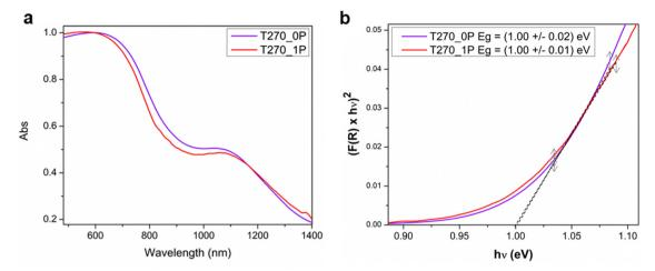
Fig. 6 (a) UV-vis absorption spectra of the T270\_0P and T270\_1P samples. (b) Tauc plot after Kubelka-Munk transformation for the direct band gap of Bi<sub>19</sub>S<sub>27</sub>I<sub>3</sub> in samples T270\_0P and T270\_1P. Calculated values are shown with the error of fitting.
