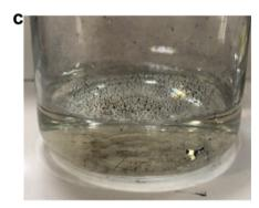
Fig. 8 (a) Sample T270\_1P suspended in Cr(vi) aqueous solution in a falcon tube; (b) sample T270\_0P suspended in Cr(vi) aqueous solution in a falcon tube; (c) sample T270\_0P in Cr(vi) aqueous solution in the photocatalysis reactor.
