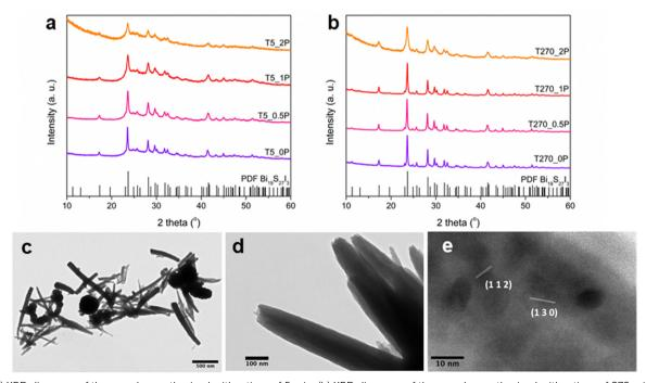
Fig. 1 (a) XRD diagrams of the samples synthesized with a time of 5 min, (b) XRD diagrams of the samples synthesized with a time of 270 min, (c) TEM image of a representative sample synthesized with PEG (T5\_1P), with nanorolls and round nanoparticle morphologies, (d) TEM image of nanorolls, and (e) HR-TEM image of a nanoroll.
