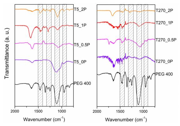
Fig. 4 FTIR spectra of the Bi<sub>19</sub>S<sub>27</sub>I<sub>3</sub> samples compared with PEG 400 for 5 and 270 minutes of reaction. The bands of interest are marked in both graphs.
