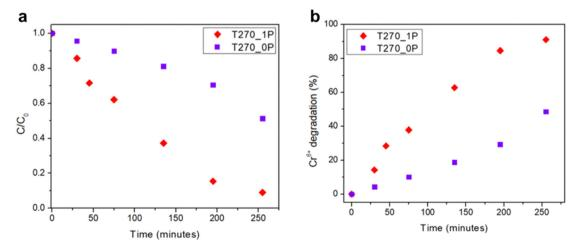
Fig. 7 (a) Cr(vi) reduction using Bi<sub>19</sub>S<sub>27</sub>I<sub>3</sub> synthesized with and without PEG as the capping agent as photocatalysts, and (b) variation in the % of Cr(vi) reduction over time
