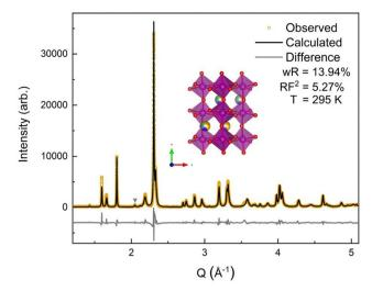
Fig. 3 SXRD pattern collected at Argonne National Laboratory's 11-BM beamline with a wavelength of 0.4582 Å. The orange circles show the collected data with the black line denoting the calculated diffraction pattern fit using the GSAS-II program, a wR of 13.94% was obtained with a main phase  $RF^2$  of 5.27%. The gray triangle denotes the impurity peak. The light gray line shows the difference curve, (data-fit) shifted down for visibility.
