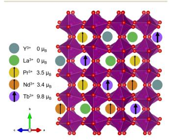
Fig. 1 Cartoon depiction of the (5A)MnO<sub>3</sub> unit cell showcasing the large variance in magnetic moment<sup>17</sup> on the A-site.
