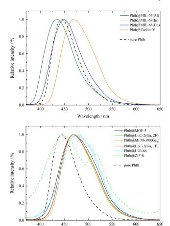
Fig. 2 Normalized emission bands of Phth embedded in different porous host matrices in comparison to pure Phth (dashed black lines). Excitation wavelength:  $\lambda_{ex}$  = 347 nm (pure Phth and **1** to **8**) and  $\lambda_{ex}$  = 340 nm (**9** and **10**).
