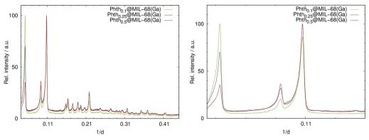
Fig. 5 Left: PXRD patterns of the serial dilution of Phth in MIL-68(Ga); right: detailed view of the low angle region of the PXRD patterns of Phth<sub>x</sub>@MIL-68(Ga) (Huber G670:  $\lambda = 1.54056 \text{ Å}$ ; 298 K)
