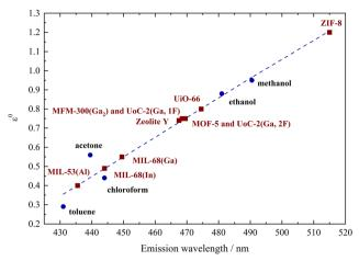
Fig. 3 Plot of the emission maxima of Phth dissolved in different solvents (blue dots) versus the elution power  $\varepsilon^0$  on alumina taken from Snyder<sup>30</sup> connected by a linear fit (blue dotted line), classifying the polarity of the respective MOFs and porous materials (red squares).
