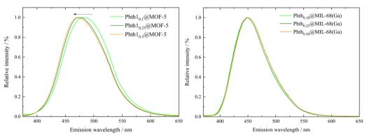
Fig. 6 Emission spectra of Phth<sub>x</sub>@MOF-5 (left) and Phth<sub>x</sub>@MIL-68(Ga) (right) with  $\lambda_{PX}$  = 347 nm.
