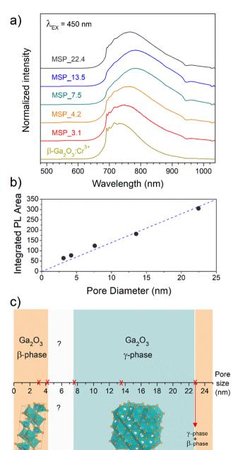
Fig. 3 (a) PL spectra of  $Cr^{3+}$  in  $Ga_2O_3$  NCs grown in mesopores of different size, (b) integrated PL area as a function of the pore size and (c) diagram of the stabilized  $Ga_2O_3$  polymorph *versus* pore size.
