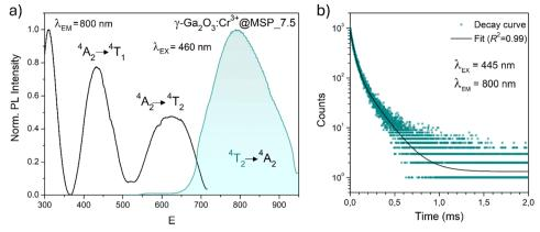
Fig. 6 PL and PLE spectra of the  $\gamma$ -Ga<sub>2</sub>O<sub>3</sub>:Cr<sup>3+</sup>@MSP\_7.5 sample after excitation at 460 nm and collecting at 800 nm, respectively. (b) Decay curve after excitation at 445 nm and collecting at 800 nm along with the fitting curve.
