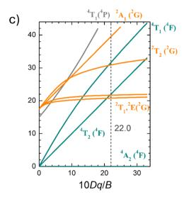
Fig. 7 (a) The PL spectrum at 80 K collected at 800 nm and (b) magnification of the (A)  ${}^4T_2$  zero phonon line and  ${}^2E$  peaks, in the energy scale. (c) Tanabe-Sugano diagram calculated for Cr3+ in γ-Ga<sub>2</sub>O<sub>3</sub> calculated considering C/B of 4.21.
