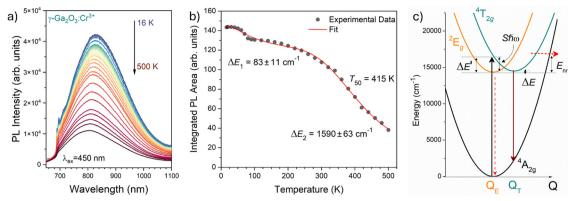
Fig. 8 (a) Temperature dependence of the PL emission spectra of  $\gamma$ -Ga<sub>2</sub>O<sub>3</sub>:Cr<sup>3+</sup> NCs from 16 to 500 K (7). (b) Temperature dependence of the integrated PL intensity (black dots) and fit (red curve). (c) Configurational coordinate diagram constructed by using eqn (5)–(7).
