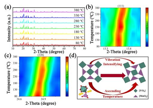
Fig. 2 Temperature-dependent (a) XRD patterns of  $Y_2Mo_3O_{12}$  and two-dimensional mapping of diffraction peaks (b) (111) and (c) (220) as well as (d) lattice distortion diagram of  $Y_2Mo_3O_{12}$ .
