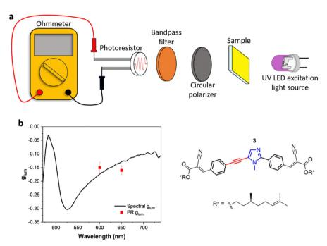
Fig. 2 (a) Experimental setup of optical and electronic components involved in ultra-cheap CPL detection. (b) Graphical representation of  $g_{lum}$  values obtained through photoresistor detection (PR  $g_{lum}$ ) in comparison with the spectral  $g_{lum}$  obtained with a standard benchtop CPL spectropolarimeter. The error bars reported for the PR  $g_{lum}$  values represent the standard deviation over a set of measurements.
