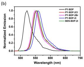
Fig. 1 (a) Normalized UV-vis absorption spectra, and (b) normalized fluorescence emission spectra of the prepared compounds in toluene ( $c = 1.0 \times 10^{-5}$ )  $10^{-5}$  M, T = 25 °C).
