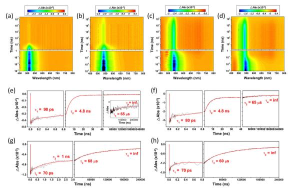
Fig. 7 Fs-to-µs TA 2D map of (a) PY-BDP, (b) PY-BDP-2CI, (c) PY-BDP-2Br, and (d) PY-BDP-2I in toluene under photoexcitation at 500 nm. TA decay profiles of (e) PY-BDP, (f) PY-BDP-2CI, (g) PY-BDP-2Br, and (h) PY-BDP-2I at 505, 535, 535, and 540 nm, respectively. Because our measured time window, 240 µs, is not enough to measure the longest decay time constant, we estimated the other time constants with the last infinite time constant.
