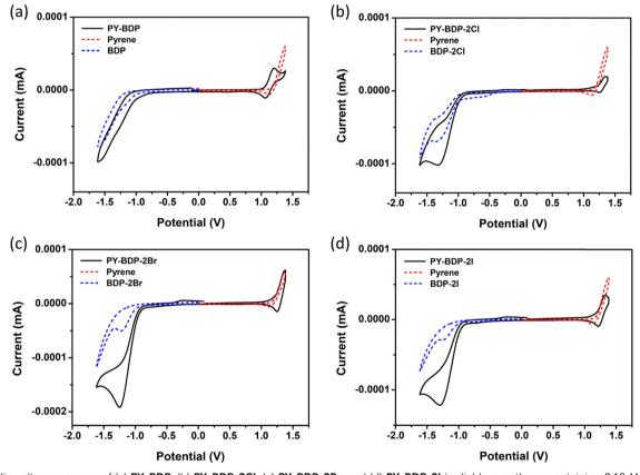
Fig. 5 Cyclic voltammograms of (a) PY-BDP, (b) PY-BDP-2CI, (c) PY-BDP-2Br, and (d) PY-BDP-2I in dichloromethane containing 0.10 M Bu<sub>4</sub>NPF<sub>6</sub> as the supporting electrolyte and Ag/AgCl as the reference electrode. Ferrocene (Fc) was used as the external reference ( $E_{1/2} = +0.38 \text{ V}$ , Fc<sup>+</sup>/Fc) (scan rate = 100 mV s<sup>-1</sup>,  $c = 1.0 \times 10^{-3} \text{ M}$ ,  $T = 25 \,^{\circ}\text{C}$ ).
