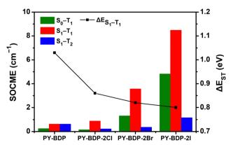
Fig. 4 Calculation of the magnitude of the spin-orbit coupling matrix element (SOCME) between  $S_n$  and  $T_m$  based on the type of heavy atom and the energy gap between the  $S_1$  and  $T_1$  states.
