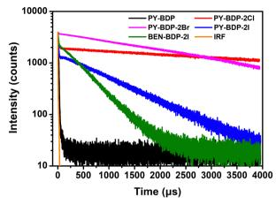
Fig. 3 Triplet–triplet annihilation delayed fluorescence of **PY-BDP**, **PY-BDP-2Cl**, **PY-BDP-2Br**, **PY-BDP-2I**, and **BEN-BDP-2I** in deoxygenated toluene was measured at 580 nm ( $c = 1.0 \times 10^{-5}$  M, T = 25 °C).
