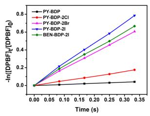
**Fig. 2** Time dependence of ln([DPBF]<sub>t</sub>/[DPBF]<sub>0</sub>) on the irradiation time in the presence of a photosensitizer and DPBF (505 nm green laser excitation).
