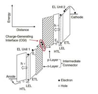
Fig. 6 Schematic of vacuum energy levels of each unit of tandem OLEDs.<sup>77</sup> Copyright 2016, WILEY-VCH Verlag GmbH.
