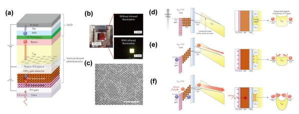
Fig. 12 (a) Schematic diagram of device structure. (b) Photos of on/off states. (c) SEM image of the porous ITO film. (d), (e) and (f) Schematic diagram of physical mechanisms.<sup>34</sup> Copyright 2016, Springer Nature.
