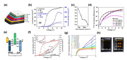
Fig. 9 (a) Schematic diagram of device structure. (b), (f) and (g) L-V & J-V characteristic curves. (c) Variation of turn-on voltage with NIR intensity. (d) Upconversion efficiency. Copyright 2019, AIP Publishing. (e) Semiconductor band diagram. (h) Digital photos of on/off states. 91,92 Copyright 2020, The Author(s).
