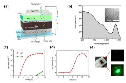
Fig. 10 (a) Schematic diagram of device structure and infrared to visible light conversion mechanism. (b) Absorption spectrum of QDs. (c) L-Vcharacteristic curves. (d) Up-conversion efficiency. (e) Schematic of on/off states. 93 Copyright 2020, SpringerNature.
