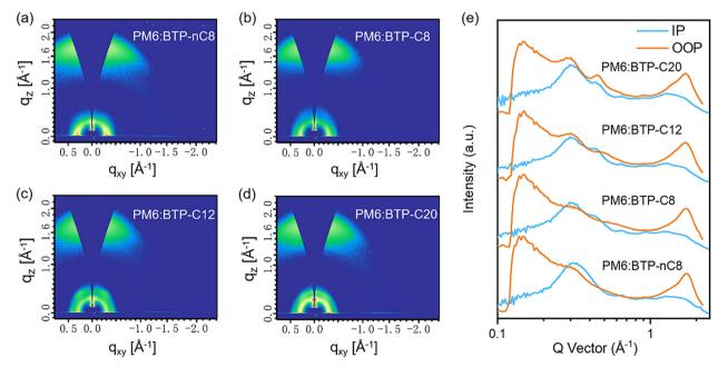
Fig. 4 (a)-(d) 2D GIWAXS patterns of the PM6:FREA blend films. (e) Corresponding GIWAXS intensity profiles along the IP and OOP directions.
