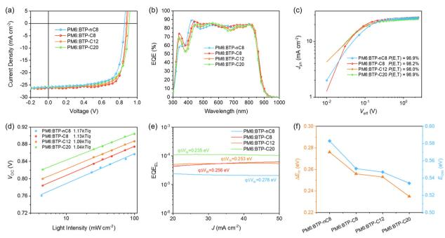
Fig. 3 (a) J-V curves and (b) EQE spectra of the optimized PM6:FREA based OSCs. (c) Photocurrent density versus effective voltage curves of the PM6:FREA based OSCs. (d) Dependence of  $V_{OC}$  on the incident light intensity of the PM6:FREA based devices. (e) EQE<sub>EL</sub> curves of the PM6:FREA based devices. (f) Comparison of  $\Delta E_{\rm nr}$  and  $E_{\rm loss}$  of the PM6:FREA based OSCs.
