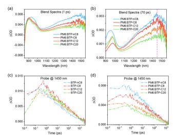
Fig. 5 Femto-TA spectra at the delay of (a) 1 ps and (b) 70 ps for the PM6:FREA blend films. fs-Resolved kinetic curves of (c) FREA neat films and (d) PM6:FREA blend films probed at 1450 nm. The fs-resolved TA data are acquired with a pump at the maximum absorption wavelength of the FREAs. The signals are normalized at the maximal amplitude of the ESA signal at 900 nm.
