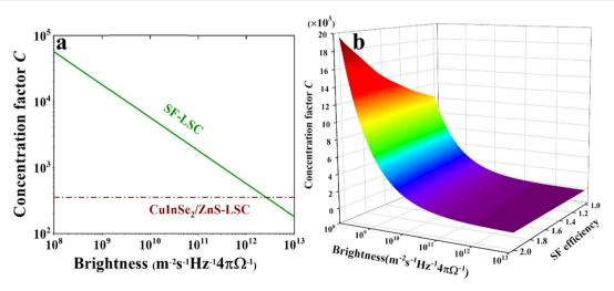
Fig. 5 (a) Thermodynamic limits of concentration factor C for NaGdF<sub>4</sub>:Yb-tetracene NC-based LSCs (green line) and CuInSe<sub>2</sub>/ZnS QD-based LSCs (red dash line) at room temperature. (b) Thermodynamic limits of concentration factor C as a function of SF efficiency and input brightness for NaGdF<sub>4</sub>:Yb-tetracene NC-based LSCs.
