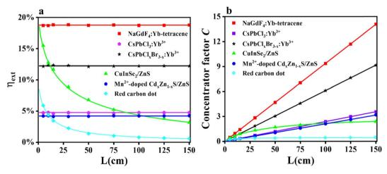
Fig. 4 Monte Carlo ray-tracing simulations of size-dependent  $\eta_{\rm ext}$  under ideal situation (a) and concentration factor C (b) for NaGdF<sub>4</sub>:Ybtetracene NCs (red curve and dots), CsPbCl<sub>3</sub>:Yb $^{3+}$  NCs (purple curve and dots), CsPbCl<sub>3</sub>Br $_{3-x}$ :Yb $^{3+}$  NCs (black curve and dots), CuInSe<sub>2</sub>/ZnS QDs (green curve and dots),  $Mn^{2+}$ -doped  $Cd_xZn_{1-x}S/ZnS$  QDs (blue curve and dots) and red CDs (cyan curve and dots).
