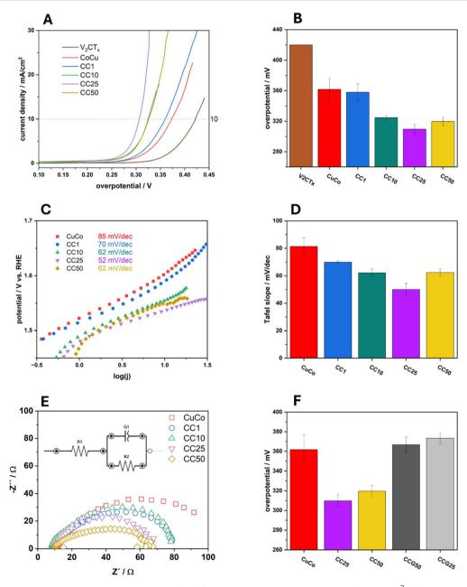
Fig. 7 (A) LSV curves of the prepared materials in 1 M NaOH (B) corresponding overpotentials at 10 mA cm<sup>-2</sup> (C) Tafel slope plots (D) corresponding Tafel slopes (E) Nyquist plots in OER region and (F) comparison to graphene composites.
