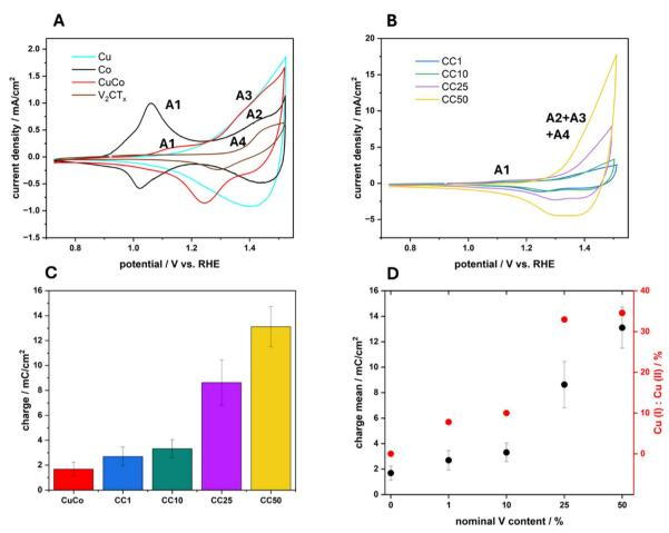
Fig. 6 Cyclic voltammograms of (A) the pure Cu, Co, CuCo and  $V_2CT_x$  materials and (B) the chemically functionalized hybrid materials CC1, CC10, CC25 and CC50, recorded at a scan rate of 40 mV in 1 M NaOH. (C) Charges for anodic sweeps and (D) charge of anodic sweep vs. Cu(i)/Cu(ii) % from XPS data.
