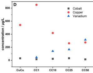
Fig. 10 XPS post-mortem analysis for the pure CuCo and CC50 catalysts at (A) Cu 2p (B) Co 2p (C) O 1s and V 2p core levels and (D) ICP-OES measurements of the electrolyte used after OER stability tests.
