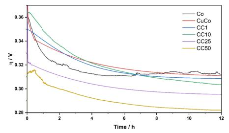
Fig. 8 Stability performance of the pure and CC materials at 10 mA cm<sup>-2</sup> over 12 hours.
