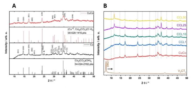
Fig. 3 (A) XRD pattern of pure Co and pure CuCo (B) XRD pattern of V<sub>2</sub>CT<sub>X</sub>, CuCo, CC1, CC10, CC25 and CC50. (\* = peak not in corresponding reference pattern).
