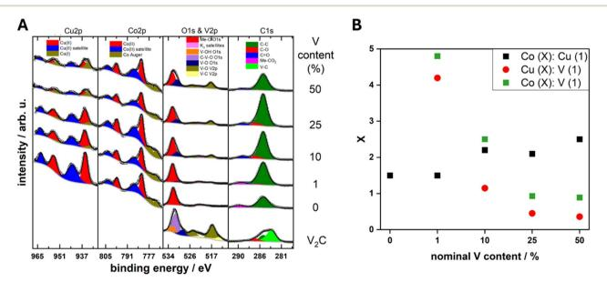
Fig. 5 (A) XPS core levels of the V<sub>2</sub>CT<sub>x</sub>, CuCo, CC1, CC10, CC25 and CC50 and (B) estimated ratios of the surface Co: Cu, Cu: V and Co: V content from XPS core level areas.
