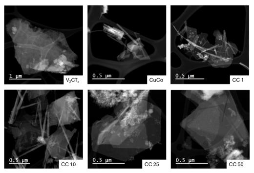
Fig. 2 HAADF-STEM images of V<sub>2</sub>CT<sub>X</sub>, CuCo, CC1, CC10, CC25 and CC50.
