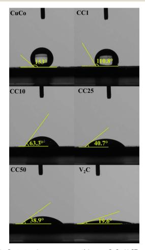
Fig. 9 Contact angle measurements of the pure CuCo, V<sub>2</sub>CT<sub>x</sub> and CC materials.
