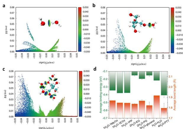
Fig. 2 Visual analysis of intermolecular interactions, (a) 1H<sub>2</sub>O–1H<sub>2</sub>O, (b) 1PTT–1H<sub>2</sub>O, and (c) 1PTT–4H<sub>2</sub>O. Color code: red, O; white, H; cyan, C. (d) Average binding energy and average H-bond length between water molecules and alcohol-based additives from theoretical calculation, including methanol (MeTH), ethanol (ETH), PP, glycerol, EG, PG, and PTT.
