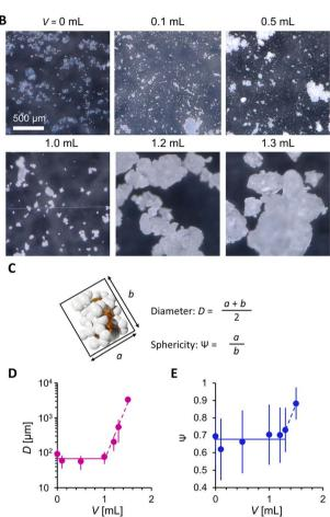
Fig. 2 (A) PDMS volume effect on PG. (B) Digital microscopic images. (C) Scheme explaining PG geometry analysis. (D) Diameter and (E) sphericity of PG. (F) Mechanical shape reconfiguration of PG.
