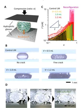
Fig. 4 (A) Scheme of the compression test. (B) Side view of the compressed PGLM just before breakage with 10  $\mu$ L water. (C) Compression–resilience curve of the PGLM with 10  $\mu$ L water in different PDMS volumes. Resilience fluctuation region (pink highlighted) is owing to the PG reconfiguration. (D) Side-view microscopic image monitoring the deformation of the PG (V=1.2 mL) during the deformation of the PGLM by a glass plate. The observed PG deformed by around 29% in height.
