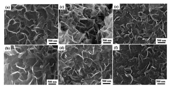
Fig. 2 FE-SEM images of VAGNAs from the pyrolysis of different biomasses with K<sub>2</sub>CO<sub>3</sub> at 1000 °C: (a) VAGNA-S-1000, (b) VAGNA-G-1000, (c) VAGNA-T-1000, (d) VAGNA-P-1000, (e) VAGNA-L-1000 and (f) VAGNA-R-1000.
