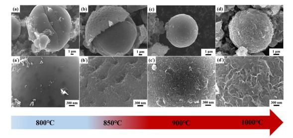
Fig. 8 Low- and high-magnification FE-SEM images of hydrothermal-treated lotus pollen-derived VAGNAs pyrolyzed with K₂CO₃ at different temperatures: (a and a') 800 °C, (b and b') 850 °C, (c and c') 900 °C and (d and d') 1000 °C.
