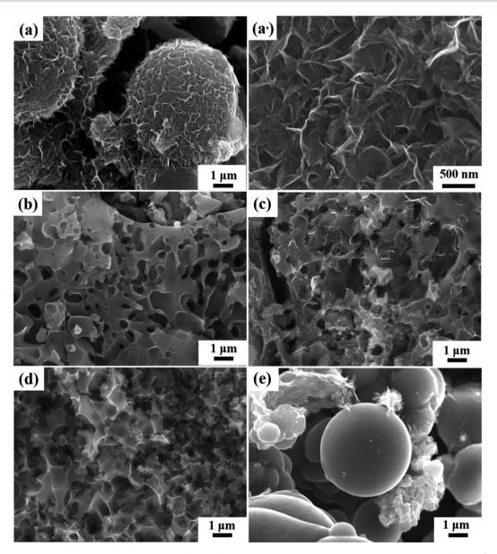
Fig. 6 FE-SEM images of lotus pollen-derived carbons (VAGNA) from pretreated precursors with different methods. (a and a'): hydrothermal treatment, (b) NaOH soaking, (c)  $H_2SO_4$  soaking, (d) ammonia soaking and (e) without pretreatment.
