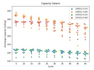
Fig. 9 A comparison of the capacity degradation of selected cells in the two cell batches assembled using Aurora, with one batch (231012) tested in-band using AiiDAlab-Aurora, and the second batch (230511) tested out-of-band of AiiDA, using EC-Lab. Only two of the four sub-batches of cells shown, a plot of all retrieved data is available in the ESI, see Fig. S6.†
