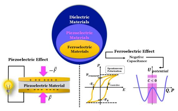
Fig. 9 Dielectric, piezoelectric, and ferroelectric materials and devices. Force  $\vec{F}$ , polarization P, capacity Q, electric field E, potential energy U, and capacitance C, remanent polarization  $P_{\text{remanent}}$ , and coercive electric field  $E_{\text{coercive}}$ .
