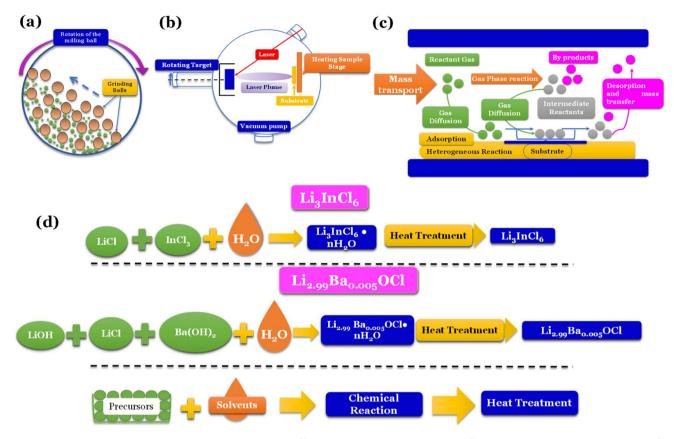
Fig. 5 Synthesis methods: (a) high energy density ball milling;<sup>76</sup> (b) pulsed laser deposition (PLD);<sup>77</sup> (c) chemical vapor deposition (CVD);<sup>78</sup> (d) water mediated synthesis of Li<sub>3</sub>InCl<sub>6</sub>, 41 Li<sub>2,99</sub>Ba<sub>0,005</sub>OCl, 29 K<sub>2,99</sub>Ba<sub>0,005</sub>OCl and Na<sub>2,99</sub>Ba<sub>0,005</sub>OCl. 28
