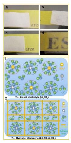
Fig. 3 Upper panel: optical image of an LC membrane (a), LC-FD membrane (b), LC membrane-based hydrogel electrolyte LC-Li<sub>2</sub>SO<sub>4</sub> (c) and LC-FD membrane-based hydrogel electrolyte LC-FD-Li<sub>2</sub>SO<sub>4</sub> (d). Lower panel: schematic diagram of the liquid electrolyte (1) and hydrogel electrolyte (2). Adapted from Qiu *et al.* (2020).<sup>42</sup> Copyright 2020. Elsevier Ltd.
