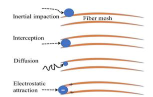
Fig. 14 Impaction, diffusion, interception, and electrostatic interaction are frequently used filtration mechanisms for biopolymers (orange lines). The pollutant, represented as a blue sphere, moves along a black path, and interactions between the pollutant and the biopolymer are shown as red dotted lines.<sup>150</sup>
