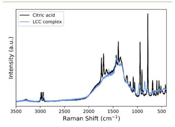
**Fig. 3** Raman spectrum of the LCC precipitate (blue) in comparison to the spectrum of citric acid (black).
