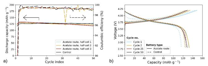
Fig. 6 Half-cell electrochemical cycling performance of NMC produced from the acetate route compared to the control NMC111 sample. (a) Discharge capacities and coulombic efficiencies of three half-cells using synthesized NMC compared to control NMC111, (b) charge-discharge profiles between 2.8 and 4.2 V for cycles 1, 2, 25, and 50 for the acetate route and the control.
