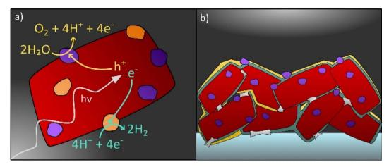
Fig. 1 Photocatalyst particle(s) (a) suspended in acidic aqueous electrolyte and (b) deposited on a conducting substrate (dark grey) forming a PEC electrode. Cocatalyst particles are coloured in orange and violet, protective layers in yellow and necking in light grey.
