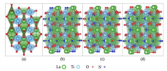
Fig. 3 (a) LaTiO<sub>2</sub>N in the orthorhombic cell observed experimentally, featuring disorder in the positions of oxygen and nitrogen. LaTiO<sub>2</sub>N (001) surface models with (b) linear *trans*-chain ordering, (c) 2D *cis*-chain ordering, and (d) mixed *trans*- and *cis*- ordering of the Ti-N-Ti bonds.
