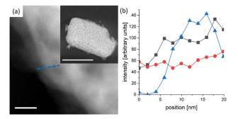
Fig. 5 LaTiO $_2$ N particle scratched from a PEC electrode after 21 h operation. (a) High angle annular dark field scanning TEM image of the edge (scale bar 20 nm) of a particle (see inset scale bar 1  $\mu$ m) (b) combined scanning TEM EDX/EELS profile along the blue line indicated in (a) triangles in blue denote N K-edge (EELS), black squares and red dots the La La and Ti K-edge respectively (EDX). The N content is reduced close to the particle edge with respect to the bulk.
