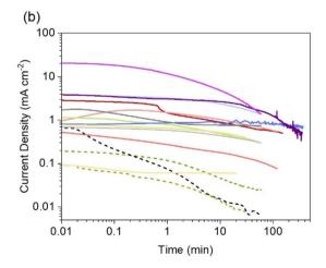
Fig. 4 Reported (photo)current densities at constant electrode potential for different systems using particle-based oxynitride photo-electrodes. (a) Data with linear axes up to 70 min, and (b) in log-scale for easier comparison between all sets of data dashed lines indicate photoelectrodes without cocatalysts. More experimental conditions, sources and colour codes can be found in Table 2.
