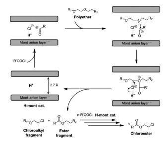
Fig. 3 Proposed catalytic cycle for the H-mont-catalysed depolymerisation of polyethers to chloroesters (reprinted with permission from Wiley, ©2016).<sup>33</sup>
