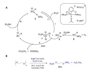
Fig. 6 (A) Proposed catalytic cycle for the of the hydrosilylation with of diethylether with the iridium pincer complex Ir-pin<sup>+</sup>. (adapted with permission from The America Chemical Society, ©2008).<sup>48</sup> (B) Reaction conditions for the iridium-catalyzed depolymerization of PEG.<sup>49</sup>
