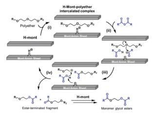
Fig. 5 Proposed catalytic cycle for the H-mont-catalysed depolymerisation of polyethers to glycol diesters (reprinted with permission from The Royal society of Chemistry, ©2017).<sup>34</sup>
