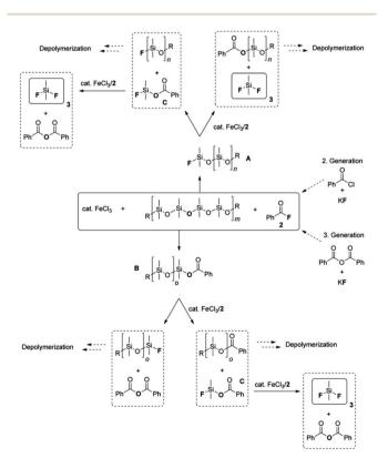
Fig. 24 Proposed mechanism for the depolymerization of PDMS catalysed by iron salts. Reprinted with permission of Wiley, © 2014.  $^{170}$
