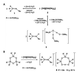
Fig. 18 (A) Equilibrium reaction of phosphazene 1, hydroxide salt 2, and silanol-silanolate salt 3; 9 (B) reaction of cyclotrisiloxanes with in situ generated phosphazenium hydroxide. Reprinted with permission from Wiley under Creative Commons License, 2019.144
