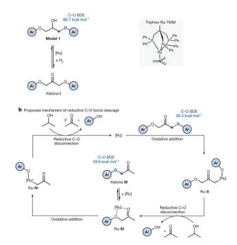
Fig. 13 (a) Concept scheme for acceptorless hydrogenation. (b) Proposed reaction mechanism for the Ru-catalysed C–O disconnection in epoxy resins and composites (adapted with permission from Springer Nature under Creative Commons licence, 2023).<sup>38</sup>
