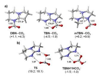
Fig. 2 Computed energetics of (a) adduct formation between superbases and  $CO_2$ ; and (b)  $HCO_3^-$  formation via the reaction of TBN with  $CO_2$  and  $H_2O$ . Relative Gibbs free energies computed in acetonitrile and butyl acetate are shown in parentheses (in kcal  $mol^{-1}$ ; with respect to separated reactants). Structures correspond to those optimized in acetonitrile. Selected bond lengths are in Å; dihedral angles defined by the atoms marked with asterisks are in degrees.
