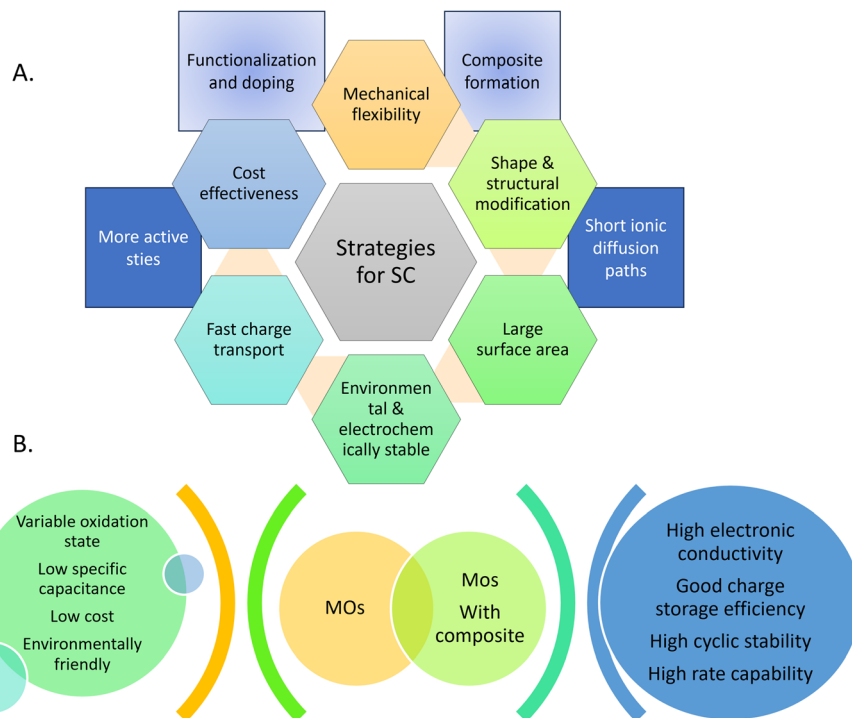
Fig. 6 (a) Enacted strategies to improve the performance of electrode materials for high-energy supercapacitors. (b) Characteristics of metal oxides and metal oxide composites in SC.
