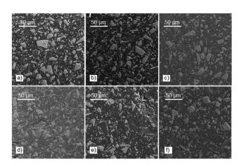
Fig. 8 SEM images showing the microstructure of the composites containing: (a) feldspar; (b) OS; (c) OS@MEMO; (d) OS@AEAPTMS; (e) OS@APTMS; and (f) OS@ODTMS.
