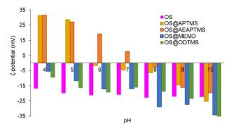
**Fig. 3** ζ-Potential of native OS (pink), OS@APTMS (33 600 ppm Si) (yellow), OS@AEAPTMS (15 530 ppm Si, orange), OS@MEMO (13 600 ppm Si, blue), and OS@ODTMS (15 270 ppm Si, green), as a function of pH. All the measurements were performed in triplicate (Table S5†) with a constant conductivity of 700 μS cm $^{-1}$ .
