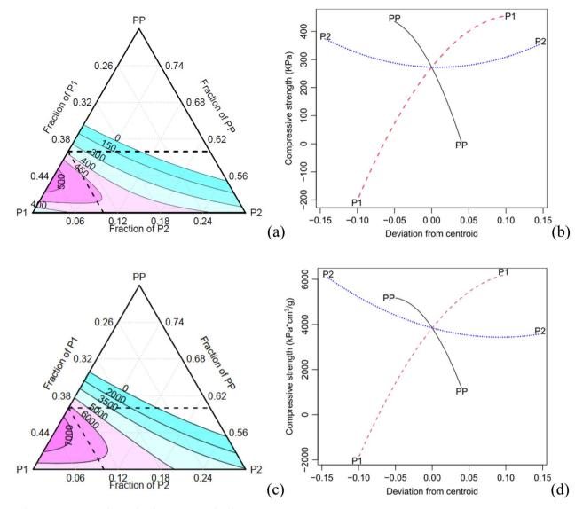
Contour and effect (plots: (a, b) absolute and(c, d) specific compressive strength.
