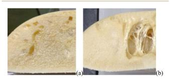
Fig. 3 Manufacturing defects obtained for (a) C3 and (b) C6, C7 conditions.
