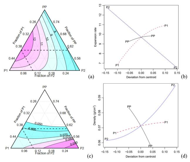
Contour and effect plots: (a, b) expansion rate and (c, d)bulk density
