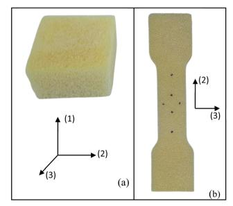
Compressive (a) and tensile (b) foam samples
