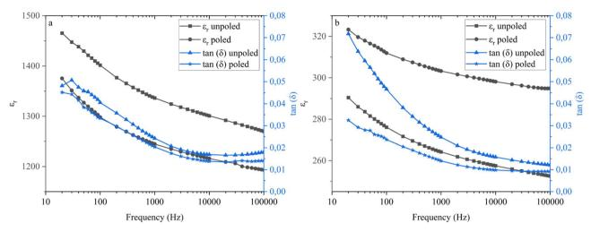
Fig. 3 Dependence of relative permittivity ( $\varepsilon_r$ ) and dielectric loss (tan( $\delta$ )) on frequency for unpoled and poled (a) BT-P and (b) BT-C measured at room temperature in the dark
