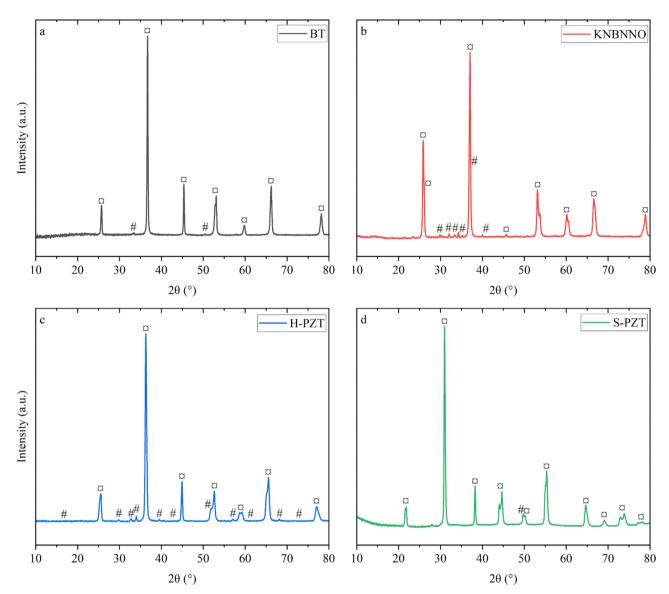
Fig. 1 XRD reflections of piezoceramic fillers: (a) BT, (b) KNBNNO, (c) H-PZT, and (d) S-PZT. Major perovskite phases are marked with 'ô' and secondary phases are marked with '#'.
