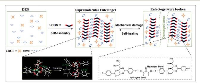
Fig. 11 Sketch of the self-healing mechanism in F-DBS-mediated supramolecular eutectogels. Reprinted from K. Fan, L. Wang, W. Wei, F. Wen, Y. Xu, X. Zhang and X. Guan, Multifunctional self-healing eutectogels induced by supramolecular assembly for smart conductive materials, interface lubrication and dye adsorption, *Chem. Eng. J.*, **441**, 136026–136034, Copyright (2022), with permission from Elsevier.
