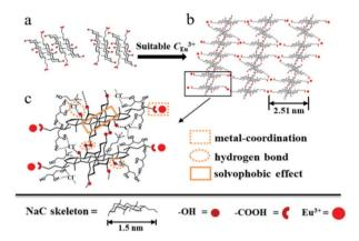
Fig. 27 Sketch of the self-assembly route and intermolecular interactions in the Eu<sup>3+</sup>/NaC/ChCl-Gly eutectogel. (a) Scheme of NaC dimers; (b and c) self-assembly of NaC/ChCl-Gly in the presence of Eu<sup>3+</sup> and details of the type of interactions. Reproduced from M. Sun, Q. Li and X. Chen, Self-assembled luminescent cholate gels induced by a europium ion in deep eutectic solvents, Soft Matter, 2021, 17, 2815-2822, with permission from the Royal Society of Chemistry.
