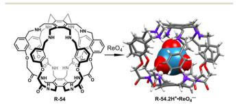
Fig. 18 Structure of receptor R-54 and the corresponding  $ReO_4^-$  binding crystal. (Data from the Cambridge Crystallographic Data Centre [CCDC # 2111255].<sup>89</sup>)
