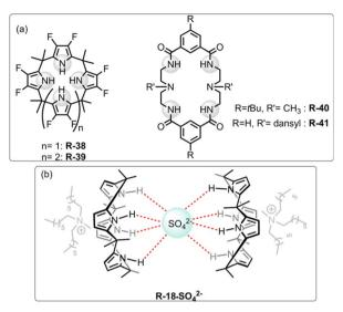
Fig. 13 (a) Chemical structure of the receptors R-38 to R-41. (b) Representation of SO<sub>4</sub><sup>2-</sup> binding with R-18.
