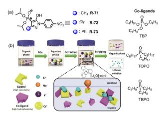
Fig. 21 (a) Chemical structure of the receptors R-71 to R-73. (b) Schematic illustration of the Li<sup>+</sup> extraction process with the presence of receptor and co-ligand. Reproduced with permission from ref. 105. Copyright 2022, Chemistry – A European Journal published by Wiley-VCH GmbH.
