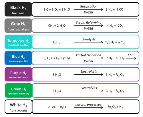
Scheme 1 Simplified chemical reactions (only one possible representative reaction is shown) associated with current fossil-based and projected hydrogen syntheses, with  $CO_2$  emissions decreasing top to bottom and the corresponding "color" scheme used in literature. WGSR: water–gas shift reaction. CCS: carbon capture and storage. <sup>78–80</sup>
