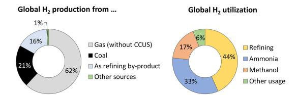
Fig. 2 Production (left) and utilization (right) of  $H_2$  in 2022, according to IEA.<sup>48</sup> "Other sources" in the  $H_2$  production panel include oil (0.5%), fossil fuels coupled to CCUS (0.6%), and water electrolysis (0.1%). "Other usage" in the  $H_2$  utilization panel is mostly linked to the iron and steel industry (DRI, Direct Reduced Iron).
