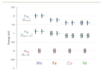
Fig. 5 Energy of 3d orbitals for  $\text{Li}_2(\text{Li}_{1-x}\text{TM}_x)\text{N}$  (where TM = Mn, Fe, Co and Ni) obtained via SA-CASSCF/NEVPT2 AILFT calculations.
