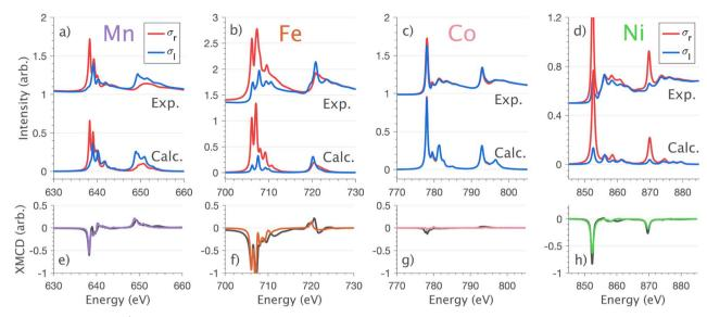
Fig. 8 Normal incidence  $(\vec{E} \pm c)$  single crystal L<sub>2,3</sub>-edge XMCD measurements and calculations of Li<sub>2</sub>(Li<sub>1-x</sub>TM<sub>x</sub>)N (where TM = Mn, Fe, Co and Ni). (a–d) Circular polarisation absorption spectra  $\sigma_r$  (red) and  $\sigma_l$  (blue) with resultant (e–h) XMCD ( $\sigma_r - \sigma_l$ ) spectra; experimental (black) and charge-transfer multiplet calculations (colour) measured at 21 K and 14 T.
