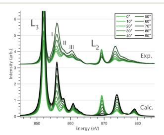
Fig. 6 Single crystal angular dependent Ni L<sub>2,3</sub>-edge XAS measurements. (Top) Experimental spectra with background subtraction. (Bottom) Charge-transfer ligand-field multiplet calculations. 0° corresponds with  $E \perp c$  and 90° with  $E \parallel c$  measured at 21 K.
