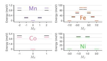
**Fig. 9** Charge-transfer ligand-field multiplet (colour) and CASSCF-QDPT-SOC. (black) Determined energy level diagrams of  $\text{Li}_2(\text{Li}_{1-x}\text{TM}_\chi)$  N exhibiting easy-planar, Mn and Co, and easy-axis, Fe and Ni anisotropy barriers to magnetisation reversal.
