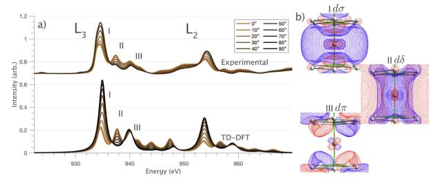
Fig. 3 (a) Single crystal angular dependent Li<sub>2</sub>(Li<sub>1-x</sub>Cu<sub>x</sub>)N L<sub>2.3</sub>-edge XAS measured at 21 K. (Top) Experimental spectra with background subtraction. (Bottom) TD-DFT calculated spectra. 0° corresponds with  $\overline{E} \perp c$  and 90° with  $\overline{E} \parallel c$ . (b) Isosurface plots of the natural transition orbitals.
