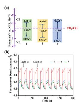
Fig. 6 (a) Energy-level diagram of 1, 3 and 4; (b) 0.4 V-bias photo-current responses of electrodes derived for 1, 3 and 4 in  $0.2 \text{ M Na}_2\text{SO}_4$  aqueous solution under repetitive chopped visible light irradiation.
