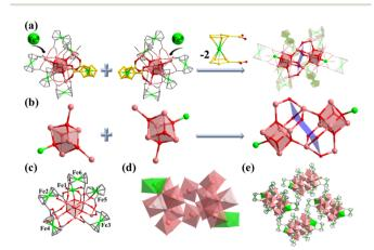
Fig. 2 Molecular structure of compound 2. (a) Assembly of the In atom in 2; (b) two cubane central ions  $[In_6Fe(\mu_4-O^{2-})_3(\mu_3-O^{2-})]^{13+}$ ; (c and d) coordination environment in 2; (e) packing structure of 2.
