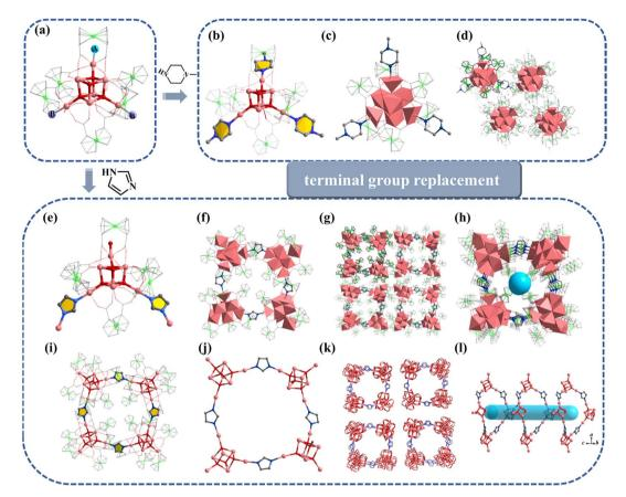
Fig. 3 Molecular structure of compound 3. (a) A and B represent substitution sites. (b and c) 3 with MPP ligand. (d) Packing of 3 along the *c*-axis. (e and f) Molecular structure of 4. (g and h) Packing structure of 4. (i–l) Cluster assembly in 4. The atom color code: pink, In; green, Fe; red, O; blue, N; gray, C; dark green, Cl.
