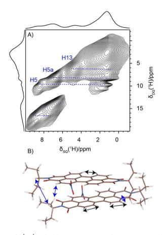
Fig. 5 (A)  $^{1}\text{H}^{-1}\text{H}$  DQ-SQ NMR spectrum of NO<sub>2</sub>-PDI collected at 60 kHz spinning speed at room temperature, using the BABA pulse sequence with a recoupling time of two rotor periods corresponding to 33  $\mu$ s. (B) Corresponding correlation is also shown.
