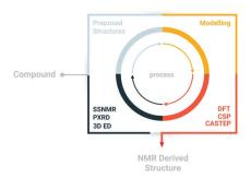
Scheme 1 Schematic diagram of the structure determination approach. The approach combines complementary techniques like powder X-ray diffraction, electron diffraction, and solid-state NMR on a quantum mechanical platform to integrate the results.
