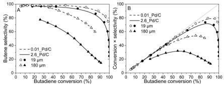
Fig. 4 Grain size affects the butene selectivity. (A) Selectivity as function of butadiene conversion of 2.6\_Pd/C (solid line, filled symbols) and 0.01\_Pd/C (dashed line, open symbols) catalysts with an average grain size of 19  $\mu$ m (circles) or 180  $\mu$ m (triangles). (B) Butenes yield during the selective hydrogenation of butadiene.
