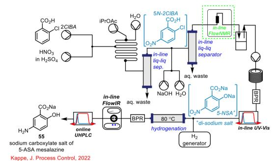
Scheme 34 Telescoped synthesis of the sodium carboxylate salt of mesalazine 55 reported by Kappe utilising in-line FlowNMR, in-line UV-vis, inline FlowIR and online UHPLC as process monitoring tools. 16,17,55
