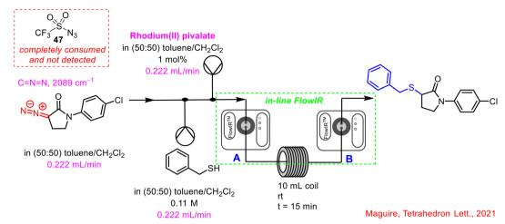
Scheme 17 Incorporation of an in-line FlowIR cell post-diazo transfer reaction and post-S-H insertion reaction by Maguire and co-workers.<sup>57</sup>
