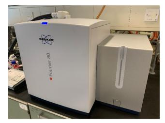
Fig. 5 Image of Bruker 80 MHz benchtop NMR spectrometer.
