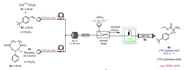
Scheme 31 In-line FlowNMR used in continuous flow cyclopropanation reaction.<sup>15</sup>
