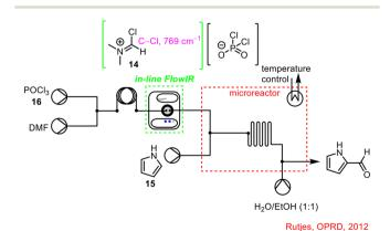
Scheme 5 In-line FlowIR flow cell used to monitor conversion of POCl<sub>3</sub> **16** in the telescoped process to synthesise 2-formylpyrrole **17** (ref. 43).
