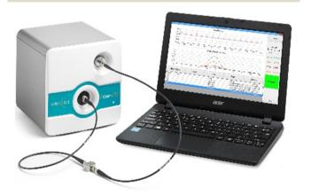
Fig. 3 Image of in-line UV-vis spectrometer by Unigsis® used in continuous flow (reproduced with permission).
