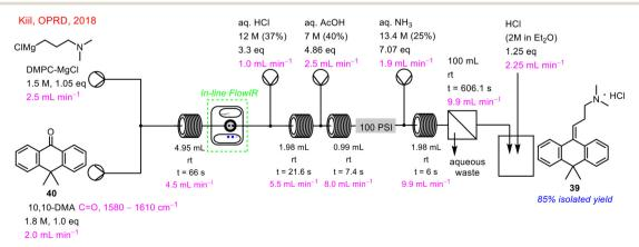
Scheme 14 In-line FlowIR in the telescoped flow synthesis of Melitracen HCl 39 (ref. 9).
