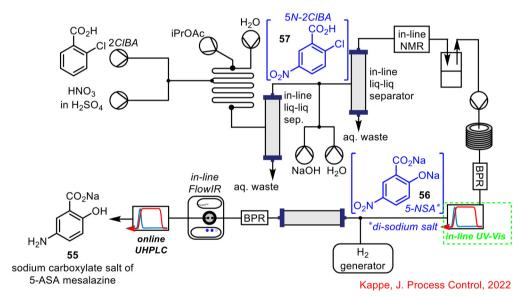
Scheme 21 Telescoped synthesis of sodium carboxylate salt of mesalazine reported by Kappe. 16,17,55
