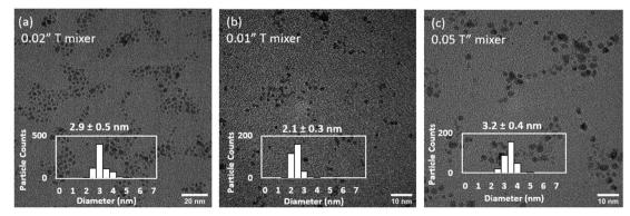
Fig. 5 Effect of internal diameter of T-mixer of (a) 0.02" (b) 0.01" and (c) 0.05" on determining early mixing rate (within 50 ms) on the size and distribution of continuously synthesised Ru NPs. Representative TEM images. Experiments 1, 4, 5, Table 3.
