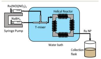
Fig. 1 Ru NP continuous reactor set up: two syringe pumps control flowrates of Ru(NO)(NO<sub>3</sub>)<sub>3</sub> and NaBH<sub>4</sub> solutions. Reactants were mixed with a T-mixer in crossflow configuration and the resulting solution passes through the coiled flow inverter reactor (CFIR).
