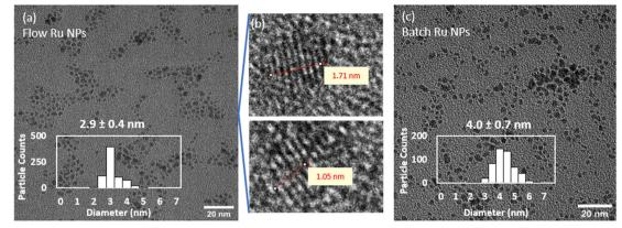
Fig. 2 Representative TEM images of (a) flow synthesis of Ru NPs collected in HNO<sub>3</sub> (b) lattice fringes from flow-synthesised Ru NPs showing spacing of 0.21 nm corresponding to hexagonal close-packed Ru(0), and (c) comparative batch synthesis. Conditions: 1.25 mM Ru(NO)(NO<sub>3</sub>)<sub>3</sub> and 3.13 mM NaBH<sub>4</sub>, pH upon mixing: 9.5, pH after HNO<sub>3</sub> quench: 1.3, 25 °C.
