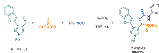
Scheme 25 Synthesis of linear carbamate derivatives by Abdou et al.
