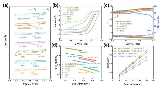
Fig. 11 Electrochemical performance of different compositions of catalysts in 0.1 M KOH  $O_2/N_2$ -saturated electrolyte using RDE. (a) Cyclic-voltammetry curves, (b) linear sweep voltammetry curves, (c) electron transfer number, n, and hydrogen peroxide yield, (d) Tafel slopes, and (e) current density as a function of scan rate at 0.4 V vs. RHE.<sup>203</sup>
