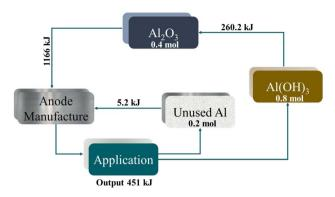
Fig. 16 Fuel energy cycle for Al-air battery applications.<sup>248</sup>
