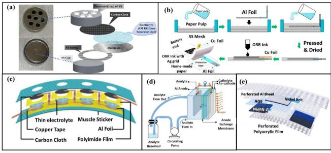
Fig. 13 (a) Coin-cell 2032-based assembly with battery components of Al-air battery. (b) Process for the fabrication of 3-D printed paperbased Al-air battery.<sup>237</sup> (c) Schematic illustration of 4 cell pack ultrathin Al-air battery made up of solid-electrolyte using aerosol jet printer.<sup>240</sup> (d) Schematic image of the dual-electrolyte system consisting of liquid anolyte and gel catholyte.<sup>242</sup> (e) Schematic illustration of AGE-based flexible wearable Al-air battery.243
