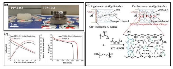
Fig. 8 (a) Optical photograph of PPM-0.3 with a weight resistance of up to 100 g. (b) Mechanical illustration of the process for the synthesis of PPM gel. (c) Electrochemical analysis with the power density and discharge curve to test the change in bent state vs. normal state of gel PPM-0.3 <sup>185</sup>
