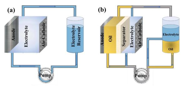
Fig. 14 (a) Schematic of conventional electrolyte with circulatory pump. (b) Oil displacement method during on/off state connected with circulatory pump.<sup>244</sup>
