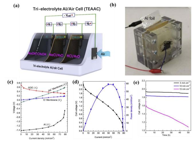
Fig. 15 (a) Schematic setup of the tri-electrolyte system of Al-air battery. (b) Camera image of the assembled Al-air cell. (c) Single-cell electrode polarization of Al, Na<sup>+</sup> membrane, Cl<sup>-</sup> membrane, and GDE. (d) Power density curve of the Al-air cell. (e) Discharge curve of Al-air cell at a current density in the range of 5-15 mA cm<sup>-2</sup>.247
