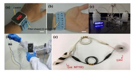
Fig. 18 Demonstration pictures of commercial LED watch operated by cabled-Al-air batteries woven into fabric from (a) front and (b) back side. <sup>187</sup> (c) Use of aqueous Al-air battery with circulating electrolyte. <sup>260</sup> (d) AGE-based flexible wearable Al-air battery showing the potential to charge a mobile phone. <sup>243</sup> (e) Ultrathin paper-based battery for powering a fan. <sup>237</sup>
