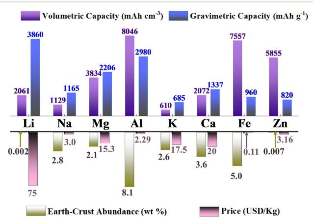
Fig. 1 A comparison of the gravimetric and volumetric capacity, Earth-crust abundance and cost of metal-anodes.
