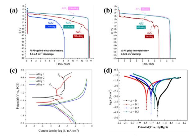
Fig. 6 (a) Galvanostatic discharge at 1.6 mA cm $^{-2}$  and (b) galvanostatic discharge at 3.2 mA cm $^{-2}$  of the Al 2024 and Al 7475 alloys in the clad and unclad states, respectively. 144 (c) Polarization curves of alloys in 2 M NaCl electrolytic solution of alloy 1-4 at 0.167 mV s<sup>-1</sup> for 30 min. 154 (d) Potentiodynamic polarization curves of the Mn-doped alloy (Al-1Zn-0.1In-0.1Sn-0.5Mg-xMn) anodes in 4 M NaOH solution at 1 mV s<sup>-1</sup> for 60 min.146
