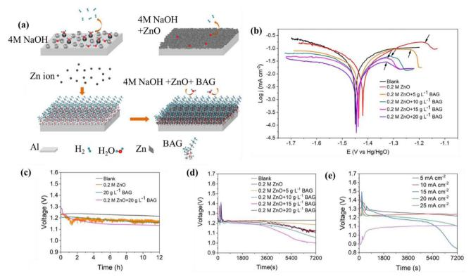
Fig. 9 (a) Schematic illustration of inhibition mechanism ZnO/BAG. (b) Polarization curves of Al in 4 M NaOH electrolytic solution with and without inhibitor. (c) Discharge curves at 20 mA cm<sup>-2</sup> for 12 h. (d) Discharge curves at 20 mA cm<sup>-2</sup> for 2 h using hybrid electrolytes. (e) Discharge curves at 10-25 mA cm<sup>-2</sup> with the hybrid of 0.2 M ZnO and 20 g per L BAG. 189
