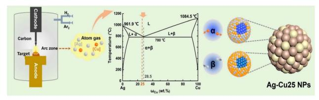
Fig. 10 Schematic illustration of the synthesis of Ag-Cu nanoparticles.<sup>203</sup>
