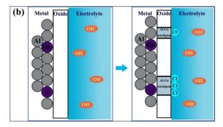
Fig. 5 (a) Schematic diagram explaining the dissolution—redeposition mechanism in Al-alloys proposed by Reboul *et al.* (b) Schematic diagram showing the eutectic mechanism.<sup>77,148</sup>
