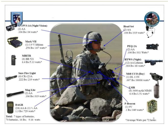
Fig. 17 Equipment carried by a soldier on a mission, with types of batteries used together with their corresponding weight and power ratings.<sup>256,257</sup>
